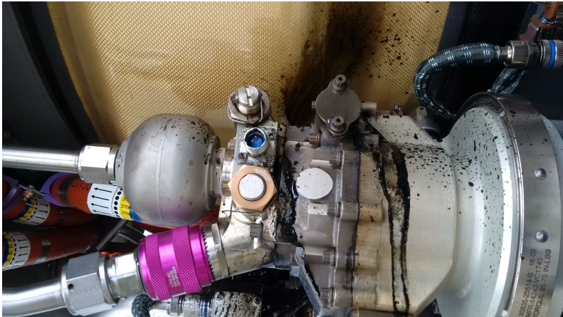
Figure 3.18: CH350's EDHP Leak.
