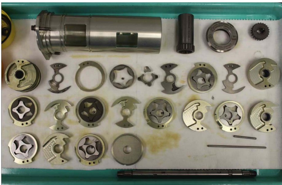
Figure 3.16: CH350's Oil Pump Component Breakdown.
