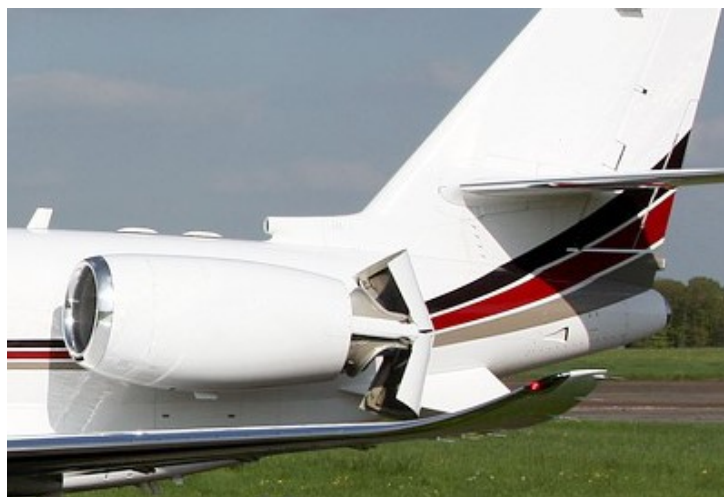
Figure 3.6: Deployed Bucket Type Thrust Reverser.
